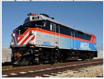
control system, remanufactured engines upgraded to U.S. EPA Tier 0+ emissions standards, new and reconditioned accessories, carbody corrosion repair and new paint, rebuilt electrical rotating equipment, rebuilt trucks with new wheels and Positive Train Control (PTC) components. Metra has assigned no. 175, the first F40PH-3, to its lines operated by Union Pacific. (RA)
