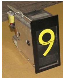
One of the “flippers” with numbers 0-9. The letter flippers had all 26 letters stored inside each!
