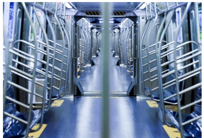
A look along the length of one of New York City Transit's new open-gangway subway trains, with no doorways between cars.
